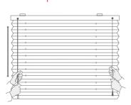
**To lower blind:** Move lift cord towards middle of the blind pulling down gently until cord lock releases.
